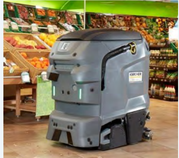
Figure 5: Adoption of robot cleaning machines requires several upstream considerations, such as minimal floor level differences and interoperability with the building infrastructure, e.g. lifts and automated doors.
